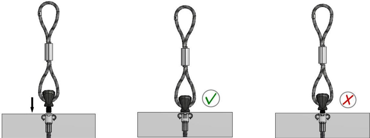
The preferred option is the vertical lift. The angle of lift ( $\beta$ ) should normally not be more than 30°. **Pulling back towards the unit is not acceptable.**
