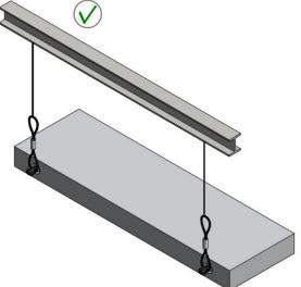
Note: Minimum radius of the crane hook for the wire loop must be **R > 1.5 x d**
