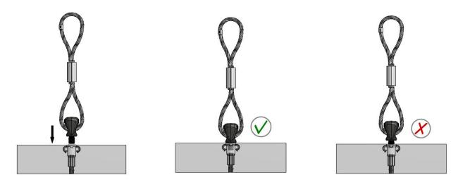
The preferred option is the vertical lift. The angle of lift (ß) should normally not be more than 30°. Pulling back towards the unit is not acceptable.
