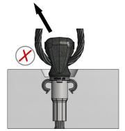
Optimum load transfer is ensured if the eye bolt is orientated in load direction.
