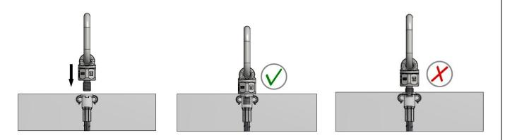
The preferred option is the vertical lift. The angle of lift (ß) should normally not be more than 30°. Pulling back towards the unit is not acceptable.
