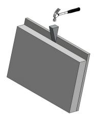
Adhesion to the formwork should be minimized before lifting the concrete element out of the formwork by removing as many parts of the formwork as possible.
