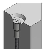
After remove the KU Nailing plate mount the plastic plug inside the socket.
