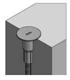
Mount the Cap in the socket after remove the Nailing plate.
