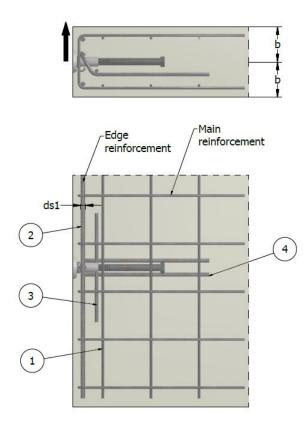
**Note:** The bending radius will be established considering the EN 1992.
