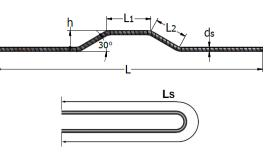
**Note:** The bending radius will be established considering the EN 1992.
