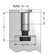
The Lifting Bolt anchor HBP is made from a threaded bush locked on a standard bolt and an anchorage plate. The threaded bush is manufactured of steel S355JO, electrolytic galvanized (EV) or hot dipped galvanized (TV), the bolt is from steel 8.8 without coating and the plate is from steel S235 also without coating.
