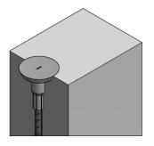
Mount the Cap in the socket after remove the Nailing plate.
