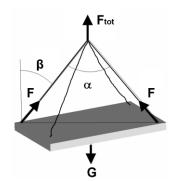
The slab unit has the following dimensions: L = 5 m, l=2m, s = 0.2 mWeight  $G = \rho \times V = 25 \times (5 \times 2 \times 0.2) =$ 50 kN Formwork area  $A = L \times l = 5 \times 2 =$  $10 m^2$
