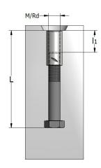
The Lifting Bolt anchors are suitable for shallow embedded elements without the need for a reinforcement tail. The force transfer into the concrete is provided by the bolt heat of the screw. For angled lifts, additional reinforcements are necessary. The lift angle must not exceed 30°. For turning/tilting a special tilting reinforcement must be used. In all cases the standard mesh reinforcement must be present into the concrete element.
