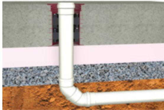
4.1.8.3 30 cm floor plate, DN/OD 160 main, DN 300 ribbed pipe
