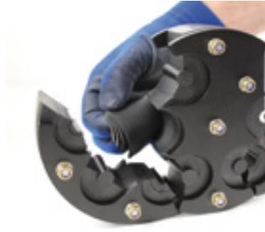
Fold back the sealing element. If required, pull out the onion rings, cut them and tear them off.
