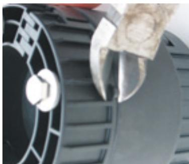
Install the sealing element as described above. For flush installation, nip off the stop lugs.
